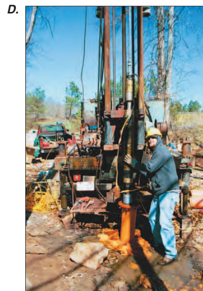
Figure 4. Down-hole packer assembly used during the study showing (A) schematic of packer assembly, and photos of (B) pressure transducers secured to top of packer assembly, (C) conductor pipe and perforated pump sleeve, and (D) lowering packer assembly into well 14FF59, Lawrenceville, Georgia.
