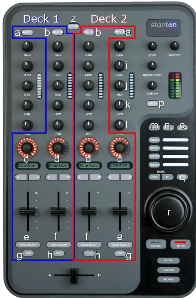
Figure68: Stanton SCS.1m (top/schematic view). Image courtesy of Stanton Magnetics, Inc., overlay (c) 2009 Sean M. Pappalardo.
