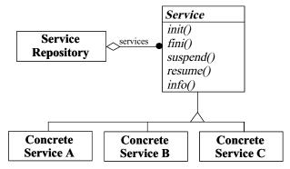
Figure 3: Structure of the Service Configurator Pattern
