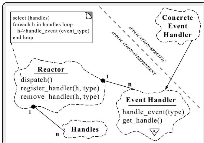
In Booch notation dashed clouds indicate classes, an inscribed “A” indicates an abstract class, directed edges indicate inheritance relationships between classes, and an undirected edge with a small bullet at one end indicates a composition relation between two classes.
