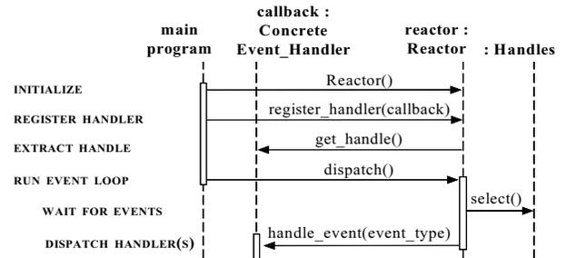
The `handle_event` method is called by the Reactor to perform application-specific functionality in response to an event. The type of the event that occurred is passed as a parameter to the method.
