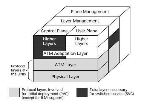
Figure 1-4 B-ISDN Protocol Reference Model
