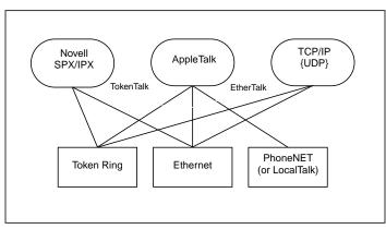
The Novel Netware<sup>®</sup> communications protocols were originally derived from the Xerox Network System (XNS) protocols. For example, the Novell Internetwork Packet Exchange (IPX) is virtually identical to the Xerox network layer protocol called IDP (Internetwork Datagram Protocol). The Novell transport protocol is called Sequenced Packet Exchange (SPX)<sup>1</sup>.
