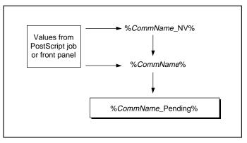
Figure 3.2 shows the basic relationship of the three parameter sets. In this figure, values written to %CommName% are written through to %CommName\_Pending%; and values written to %CommName\_NV% are written through to %CommName% and thence to %CommName\_Pending%. Beyond this, several variables exist:
