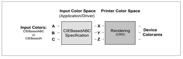
Figure 5.5 shows how the new pre-extension fits with the pre-existing **CIEBasedABC** color spaces.
