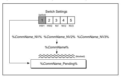
Figure 3.4 Communications parameter sets using "hard wired" values
