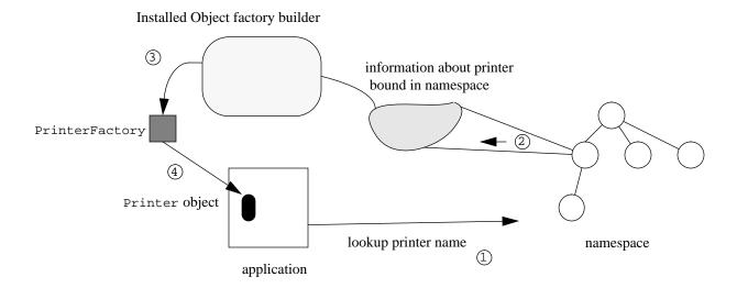
A service provider for an object factory builder must do the following:
