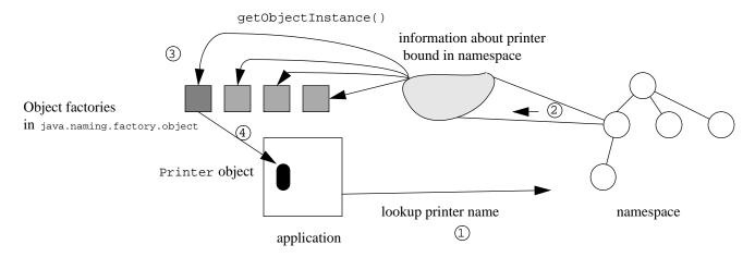
For the printer example, instead of using a Reference to represent a printer in the namespace, some other information is stored. When that information is later retrieved, the object factories specified <code>java.naming.factory.object</code> are tried in turn to attempt to turn that information into a Printer instance.
