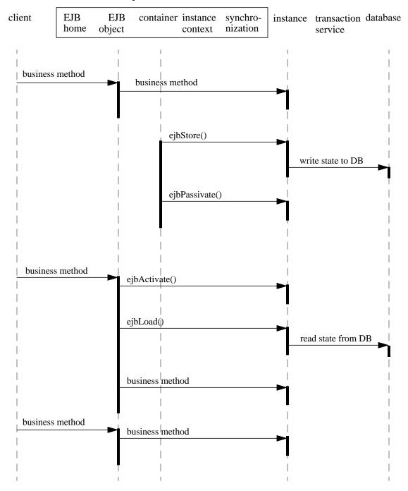
The following diagram illustrates the passivation and reactivation of an enterprise Bean instance with container-managed persistence.
