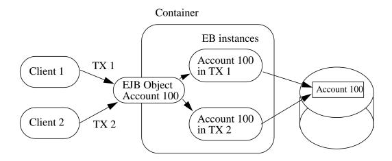
• The container acquires an exclusive lock on the instance's state in the database. The container activates a single instance and serializes the access from multiple transactions to this instance. The commit-time option A in Subsection 9.11.4 is applicable to this type of container.
