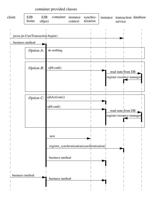
The following diagram illustrates the protocol performed for a Bean with containermanaged persistence at the beginning of a new transaction.
