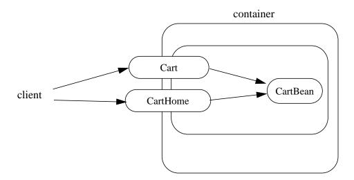
A client creates a Cart session object (which provides a shopping service) using a *create*(...) method of the Cart's home interface. The client then uses this object to fill the cart with items and to purchase its contents.
