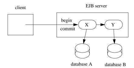
The container automatically commits the transaction at the time X returns a reply to the client.
