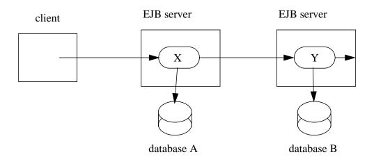
When X invokes Y, the two EJB servers cooperate to propagate the transaction context from X to Y. This transaction context propagation is transparent to the application-level code.
