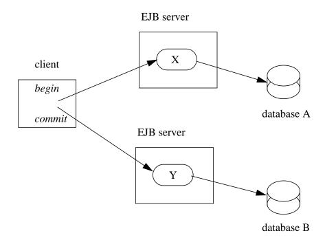
The application programmer demarcates the transaction with *begin* and *commit* calls, and the EJB server ensures that the updates to databases A and B are transactional. A proxy of a transaction service on the client automatically propagates the transaction context to the two EJB servers. When the client program calls commit, the two EJB servers perform the two-phase commit protocol.
