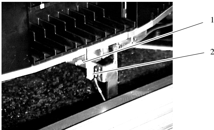
Fig. 9-56: Main Tower Reference Switch
