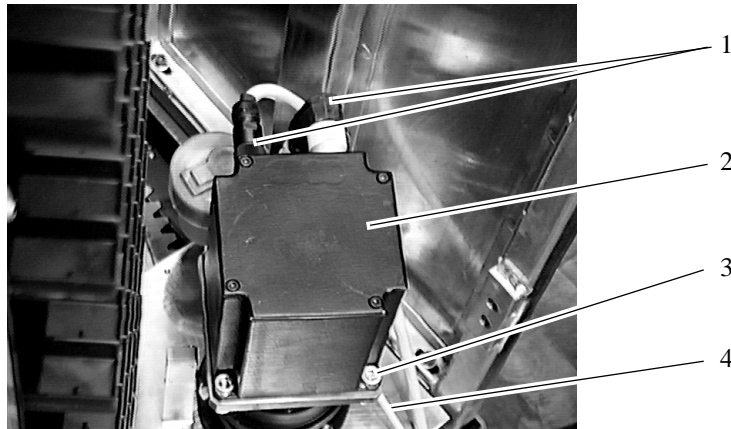
Fig. 9-52: Auxiliary Tower Drive-Motor
