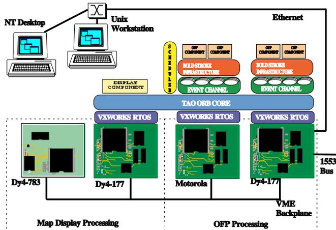
Fig. 3. Hardware and Software Configuration
