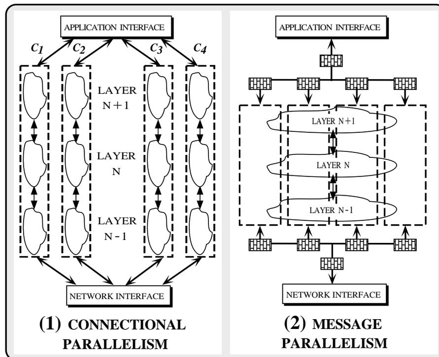
Figure 2.5: Message-based Process Architectures
