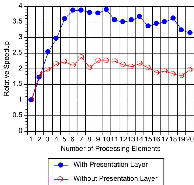
Figure 4.9: Relative Speedup for Connection-oriented Layer Parallelism
