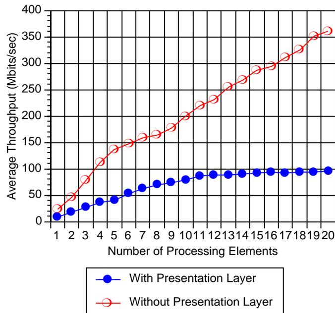
Figure 4.4: Connection-oriented Connectional Parallelism Throughput
