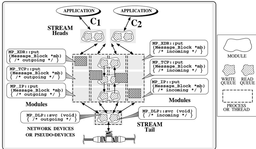
Figure 4.2: Message Parallelism Process Architecture
