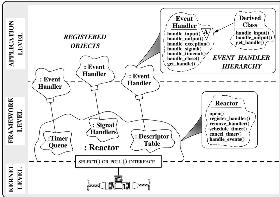
Figure 3.5: Components in the Reactor Class Category
