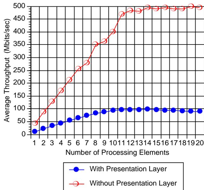
Figure 4.11: Connectionless Message Parallelism Throughput
