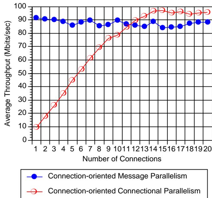
Figure 4.10: Comparison of Connectional Parallelism and Message Parallelism
