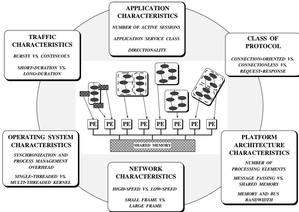
Figure 2.6: External and Internal Factors Influencing Process Architecture Performance
