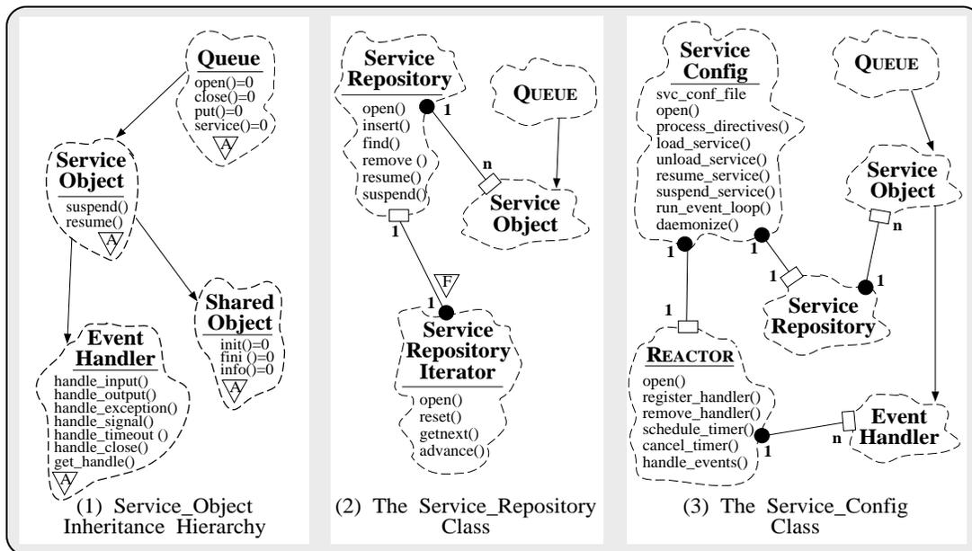
Figure 3.6: Components in the Service Configurator Class Category
