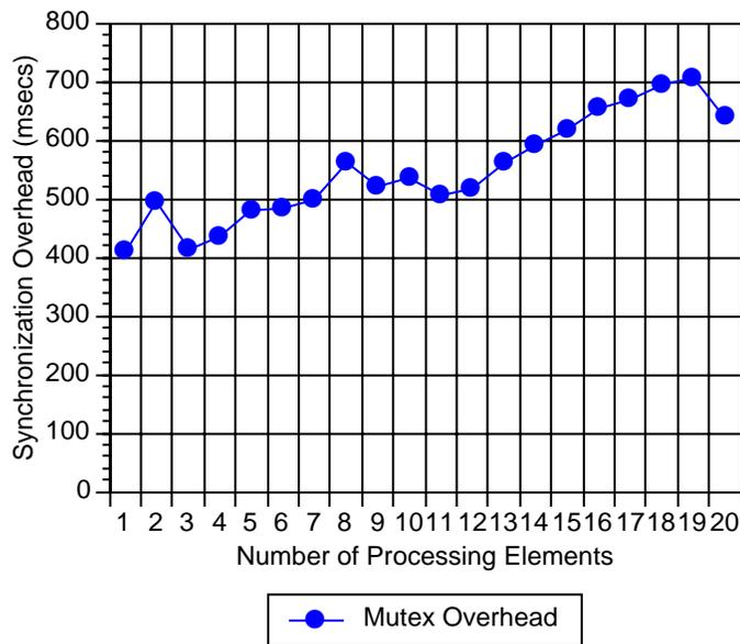
Figure 4.20: Connection-oriented Connectional Parallelism Synchronization Overhead
