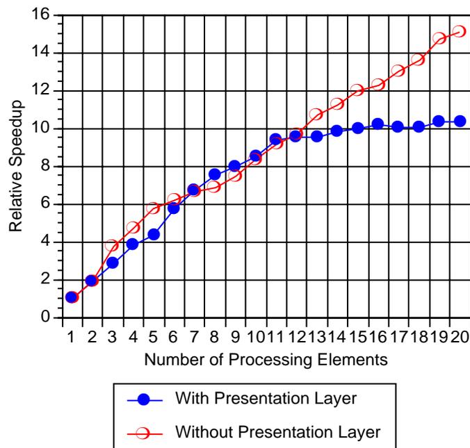
Figure 4.7: Relative Speedup for Connection-oriented Connectional Parallelism
