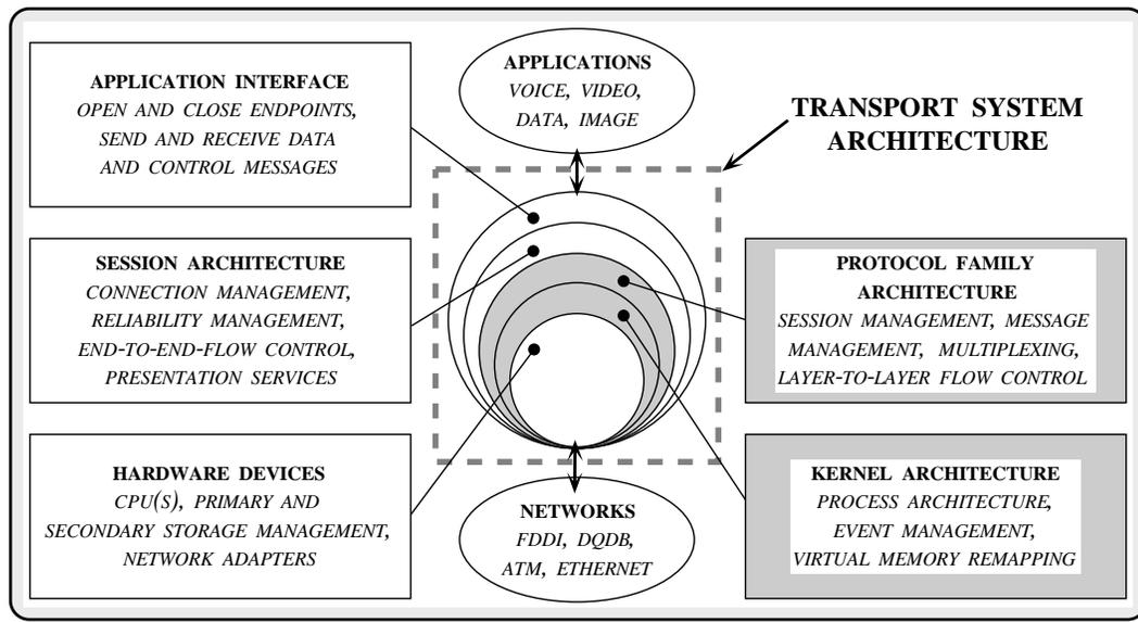
Figure 2.2: Architectural Components in a Communication Subsystem
