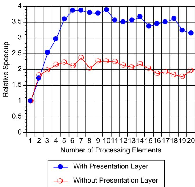
Figure 4.14: Relative Speedup of Connectionless Layer Parallelism
