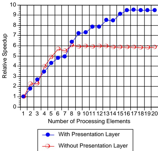
Figure 4.8: Relative Speedup for Connection-oriented Message Parallelism
