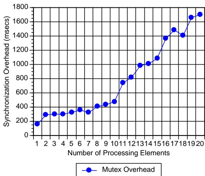
Figure 4.23: Connectionless Message Parallelism Synchronization Overhead
