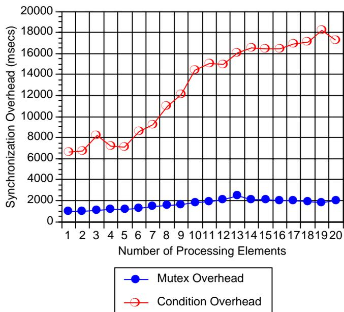
Figure 4.22: Connection-oriented Layer Parallelism Synchronization Overhead
