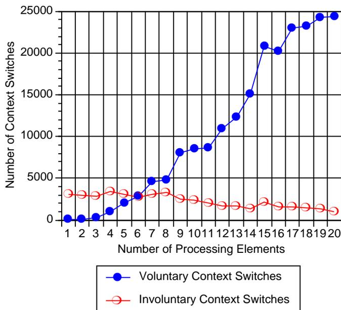
Figure 4.16: Connection-oriented Message Parallelism Context Switching
