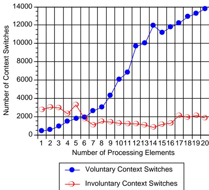
Figure 4.15: Connection-oriented Connectional Parallelism Context Switching
