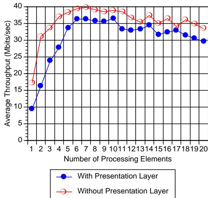
Figure 4.6: Connection-oriented Layer Parallelism Throughput
