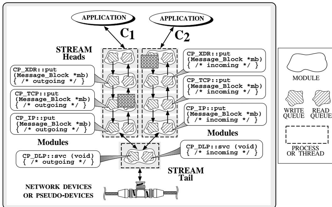
Figure 4.1: Connectional Parallelism Process Architecture
