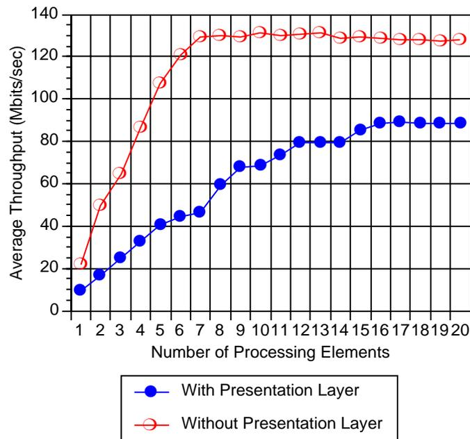
Figure 4.5: Connection-oriented Message Parallelism Throughput
