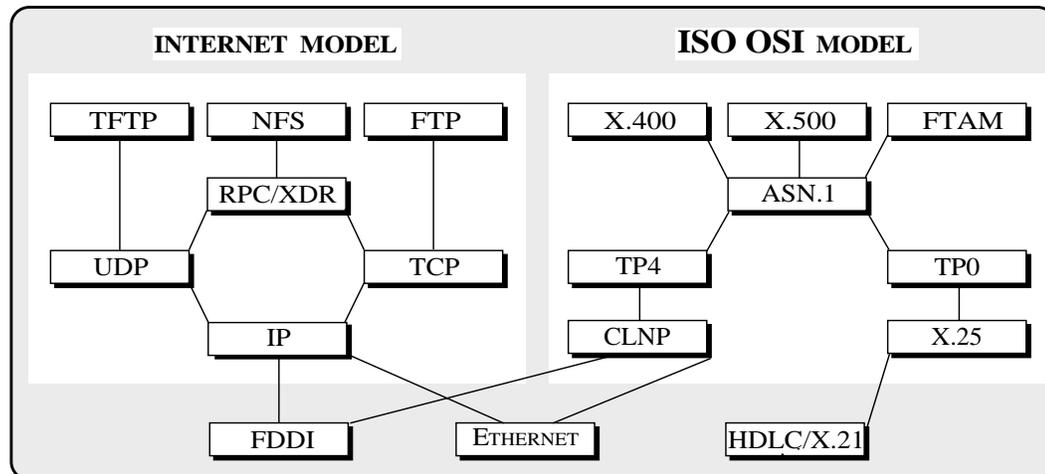
Figure 2.1: Protocol Graph for Internet and OSI Communication Models
