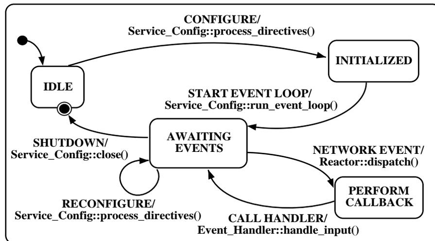
Figure 3.8: State Transition Diagram for Service Configuration, Execution, and Reconfiguration
