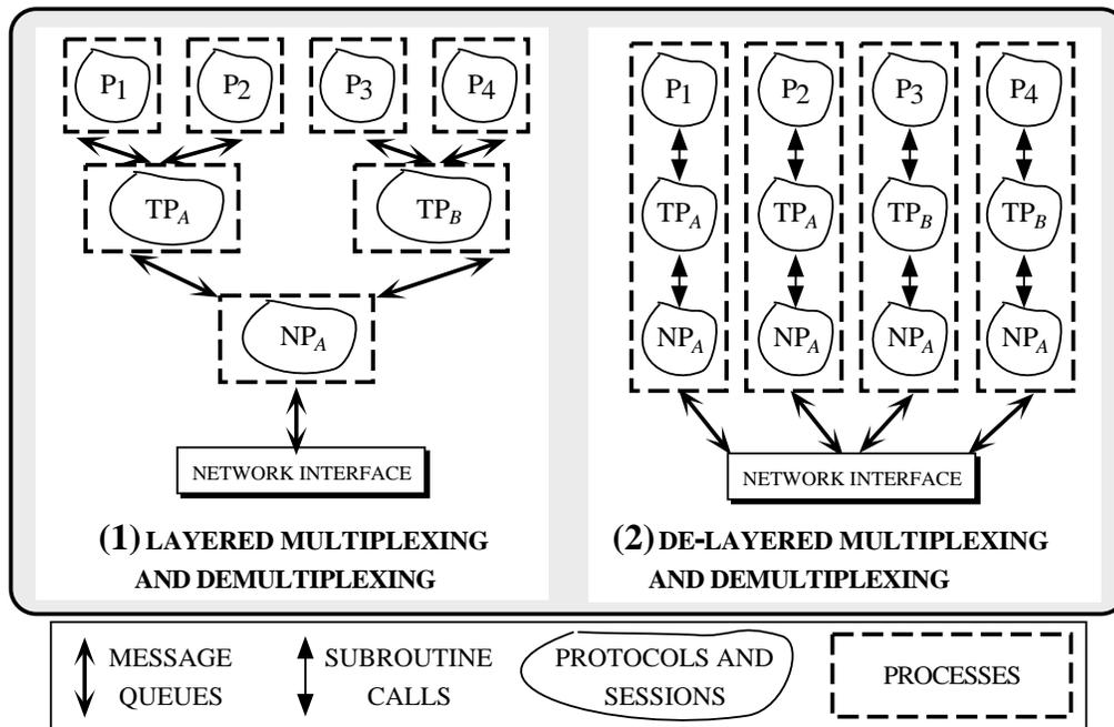
Figure 2.7: Layered and De-layered Multiplexing and Demultiplexing
