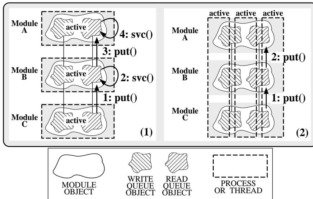
Figure 3.4: Alternative Methods for Invoking `put` and `svc` Methods
