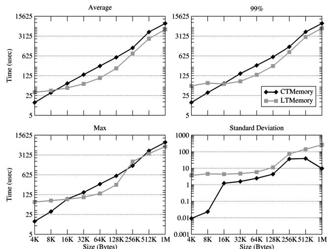
Fig. 9. Average, 99 percent, maximum, and standard deviation of the exit time ( $\mu\text{sec}$ ).
