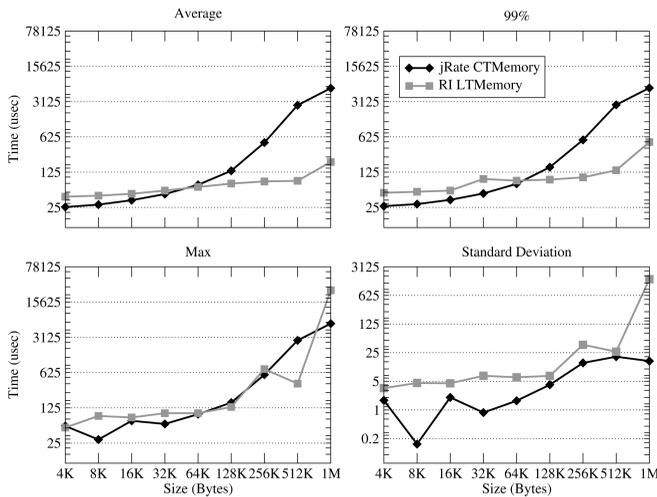
Fig. 7. Average, 99 percent, maximum, and standard deviation of the creation time ( $\mu\text{sec}$ ).
