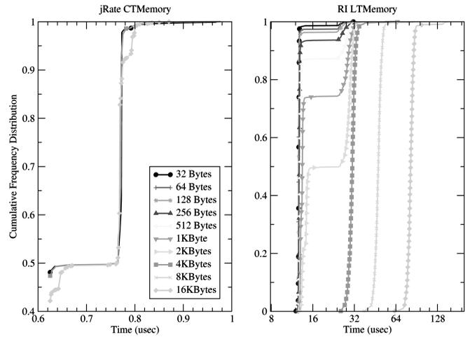
Fig. 6. Allocation time cumulative relative frequency distribution.
