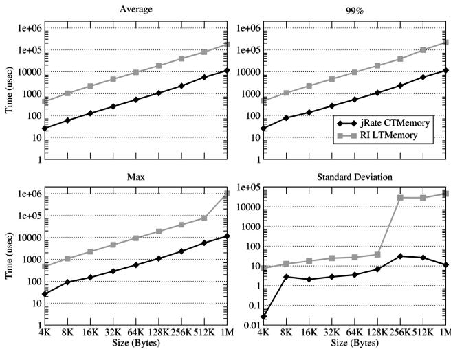
Fig. 10. Average, 99 percent, maximum, and standard deviation of the execution time ( $\mu\text{sec}$ ).
