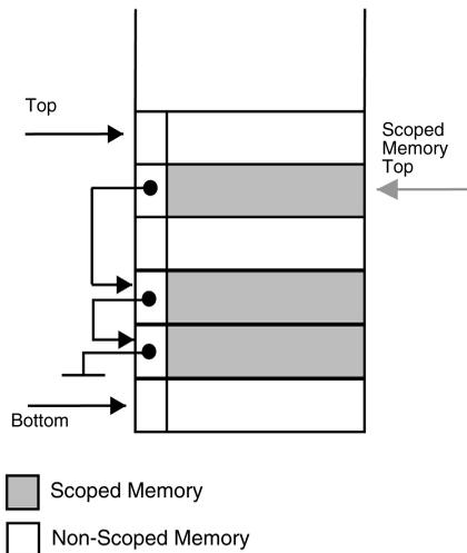
Fig. 3. The jRate scope stack structure.
