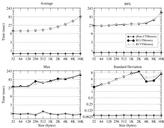
Fig. 5. Scoped memory allocation time statistics.
