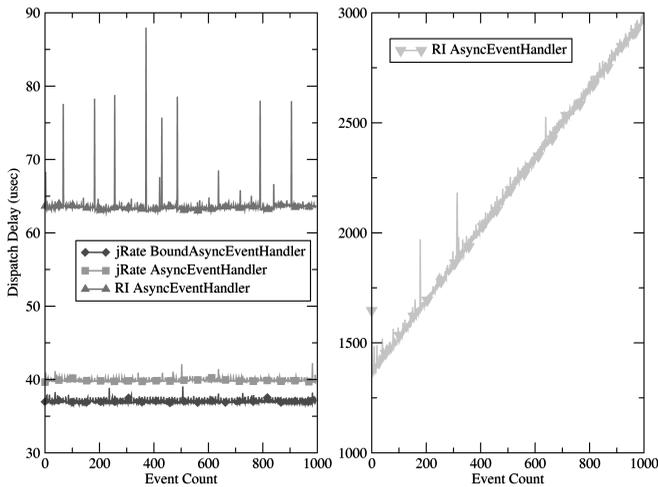
Fig. 12. Dispatch latency trend for successive event firing.
