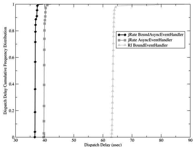
Fig. 13. Cumulative dispatch latency distribution.
