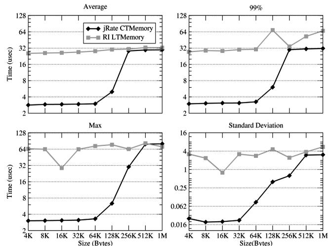
Fig. 8. Average, 99 percent, maximum, and standard deviation of the enter time ( $\mu\text{sec}$ ).
