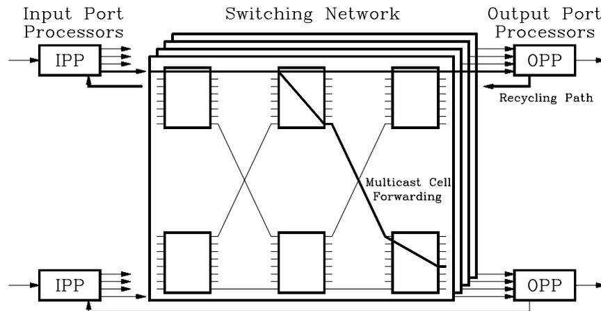
Figure 4: Gigabit ATM Switch Architecture
