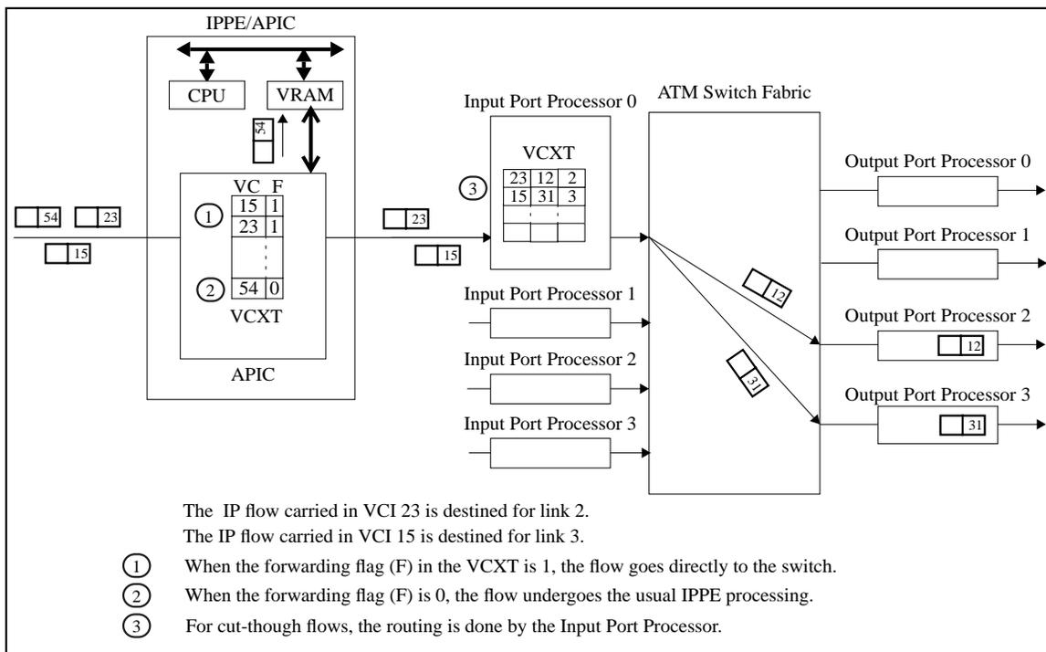
Figure 6: Cut-through Routing
