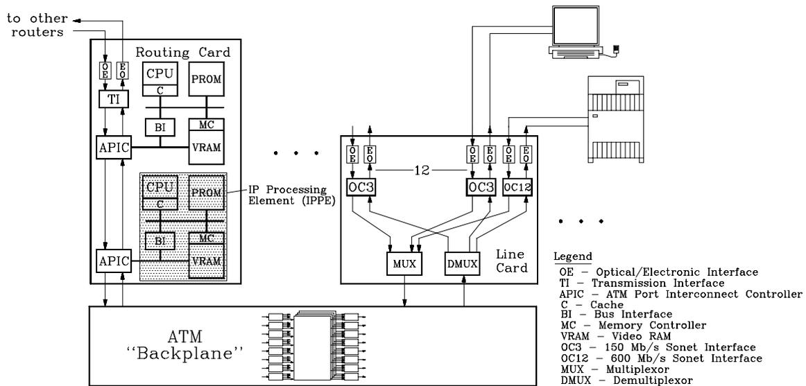
Figure 1: Gigabit a<sup>IP</sup> Router
