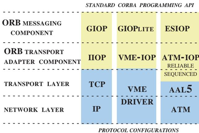
Figure 7: Relationship Between Inter-ORB Protocols and Transport-specific Mappings
