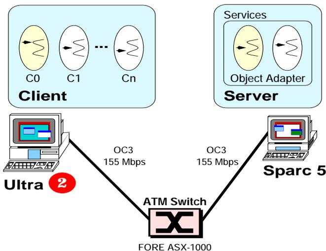
Figure 12: ORB Endsystem Benchmarking Testbed
