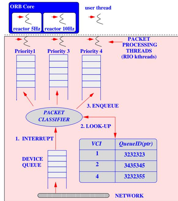
Figure 5: Early Demultiplexing in the RIO Subsystem
