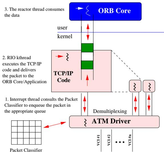
Figure 6: RIO Thread Pool Processing of TCP/IP with QoS Support
