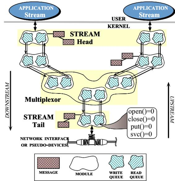
Figure 22: General Structure of a STREAM
