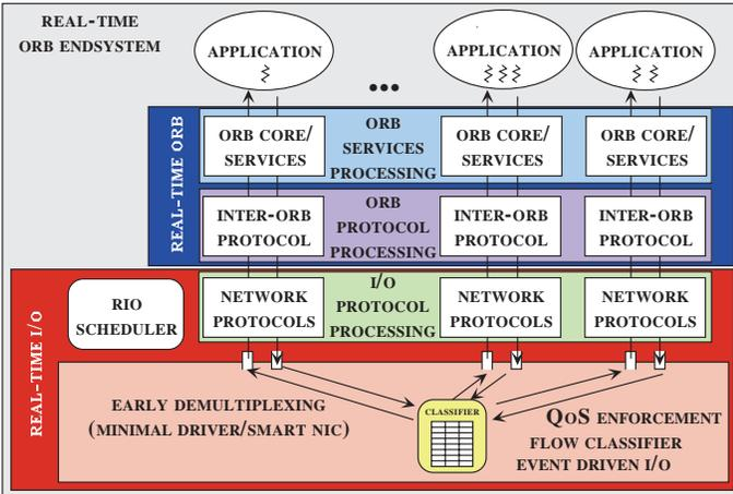
Figure 3: Architecture of a High-performance and Real-time ORB Endsystem
