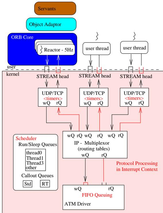
Figure 23: Conventional Protocol Stacks in Solaris STREAMS
