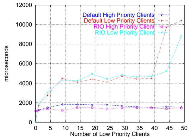
Figure 18: Measured Latency for All Clients with and without RIO
