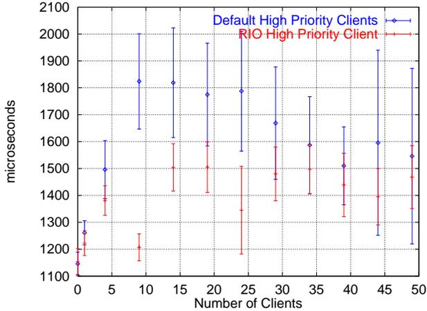
Figure 19: High-priority Client Latency and Jitter
