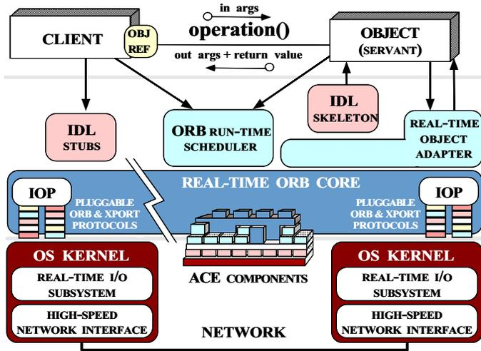
Figure 1: Components in the TAO ORB Endsistem
