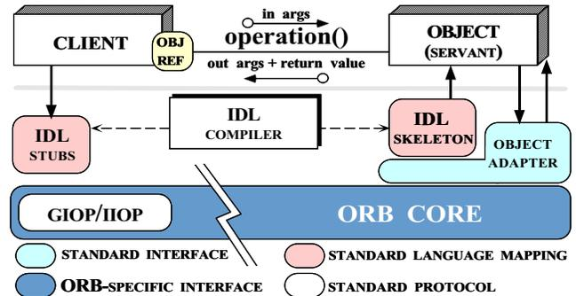
Figure 21: Key Components in the CORBA 2.x Reference Model
