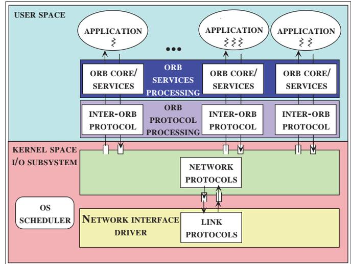
Figure 2: Typical ORB Endsysteem Architecture
