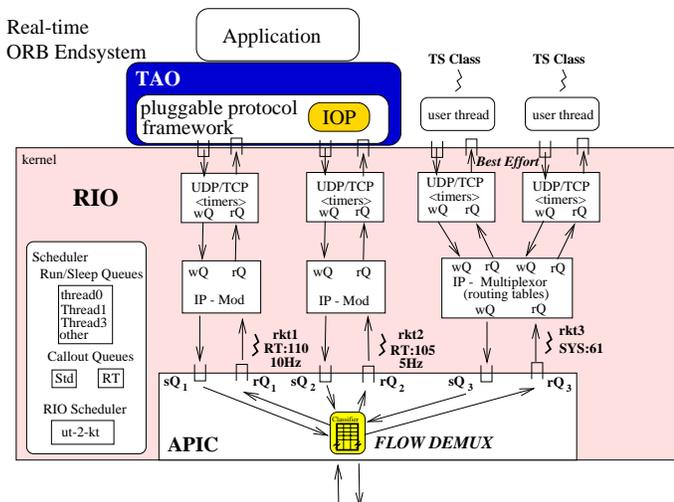
Figure 4: Architecture of the RIO Subsystem and Its Relationship to TAO
