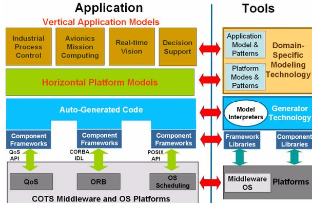
**Figure 2. MDD-Based Product-line Architecture for DRE Systems**
