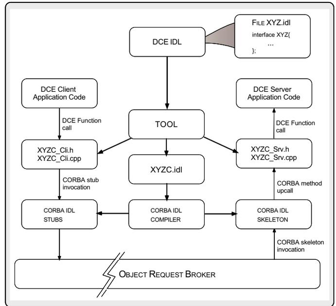
Figure 3: Interfacing Generated Code with DCE Application Code
