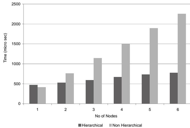
(b) Actuation Delay vs Number of Nodes
