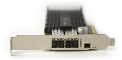
The Endace DAG® 9.2X2 is the world's first dual-port, x8 lane PCI Express 2.0 network monitoring card capable of line-rate capture to host memory on a full-duplex 10 Gigabit Ethernet link regardless of packet size (the card can alternatively be configured for full-duplex 1GbE links).
