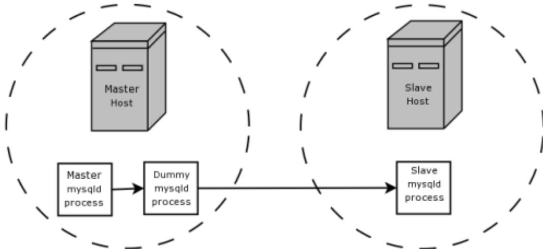
The master writes to its binary log. The “dummy” `mysqld` process acts as a slave, applying the desired combination of `replicate-do` and `replicate-ignore` rules, and writes a new, filtered binlog of its own. (See Section 6.8, “Replication Startup Options”.) This filtered log is provided to the slave.
