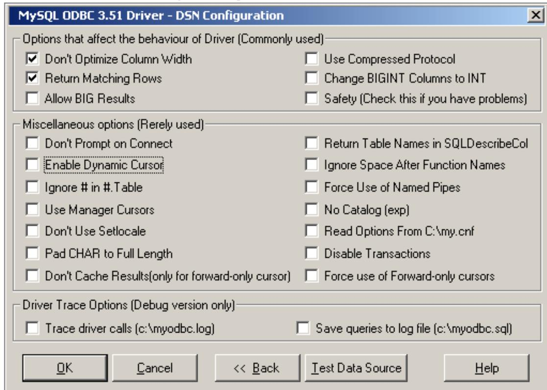
**Note:** The options listed under `Driver Trace Options` are disabled (grayed out) unless you are using the debugging version of the driver DLL.
