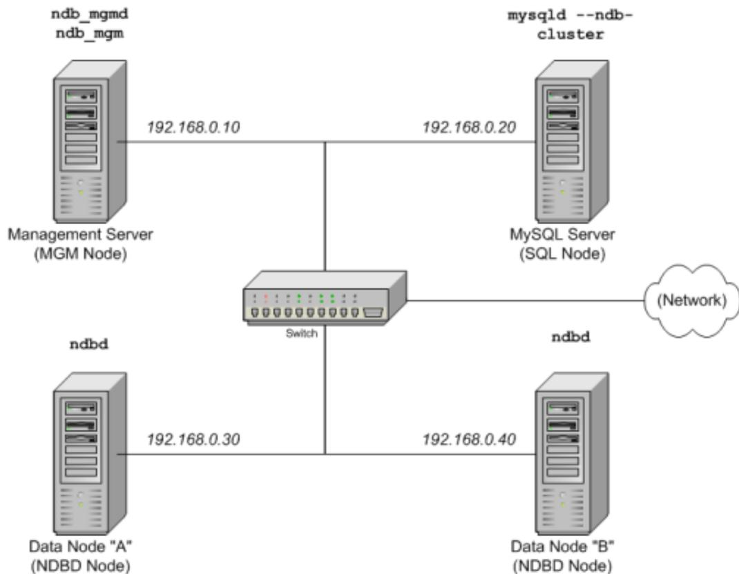
**Note:** In the interest of simplicity (and reliability), we will use only numeric IP addresses in this How-To. However, if DNS resolution is available on your network, then it is possible to use hostnames in lieu of IP addresses in configuring Cluster. Alternatively, you can also use the `/etc/hosts` file or your operating system's equivalent for providing a means to do host lookup if such is available.
